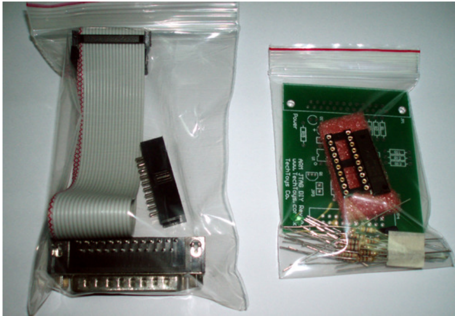
Figure 1 ARM JTAG DONGLE DIY
