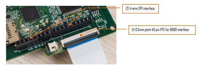
Different interface mode is selected by XPS[2:0] pins of the RA8876 illustrated by an extract from the data sheet.
