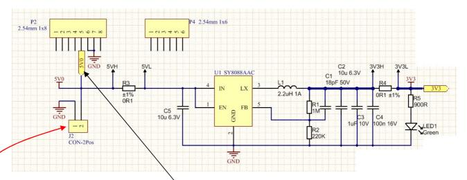
A single DC supply of 5V @ 500mA to header P2-pin5 is enough for the main power in most cases. This pin matches 5V supply of an Arduino Uno board layout, therefore it would be the USB port from your PC to supply the main power. In this case you may find your USB port slightly overloaded with 5V dropping to 4.8V or below. The overloading will be worsen when the HDMI port is connected. If 5V drops below 4.2V it is recommended to supply a regulated 5V of 500mA or above to J2.
