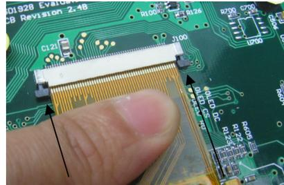
Apply pressure to these ends to lock the connector.
