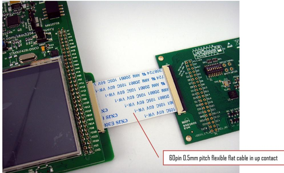
Wiring to the application module is finished with a 40pin 0.5mm pitch FFC.
