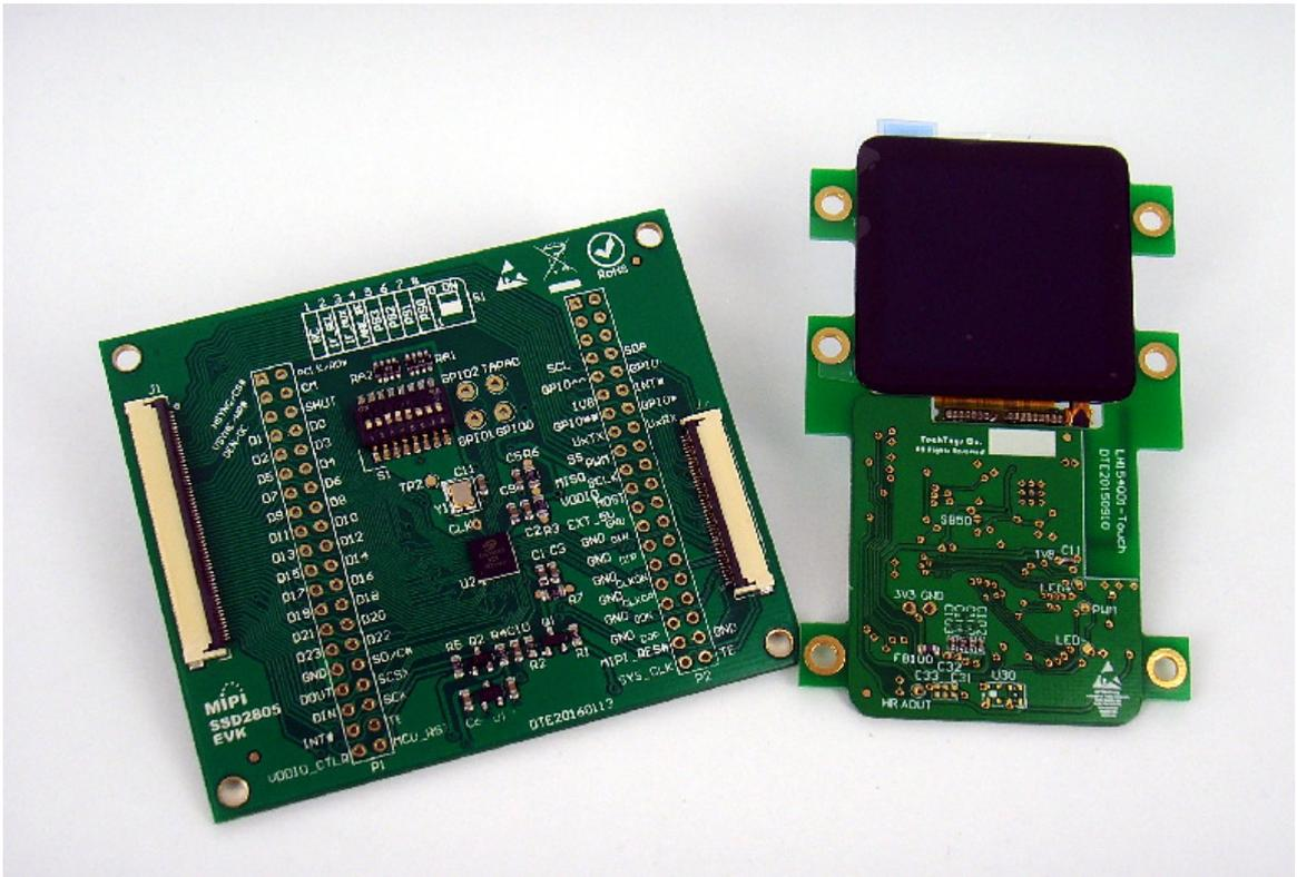
SSD2805 MIPI Master Bridge breakout board has been routed with simplicity in mind. Pixel data from an application processor (MCU/MPU) in RGB/8080 data bus is fed to the 60 pin FPC connector J1 from the left. After conversion and protocol translation finished by SSD2805, differential signals that conform to DSI specification is output through a 40 pin FPC connector J2 at the right.
