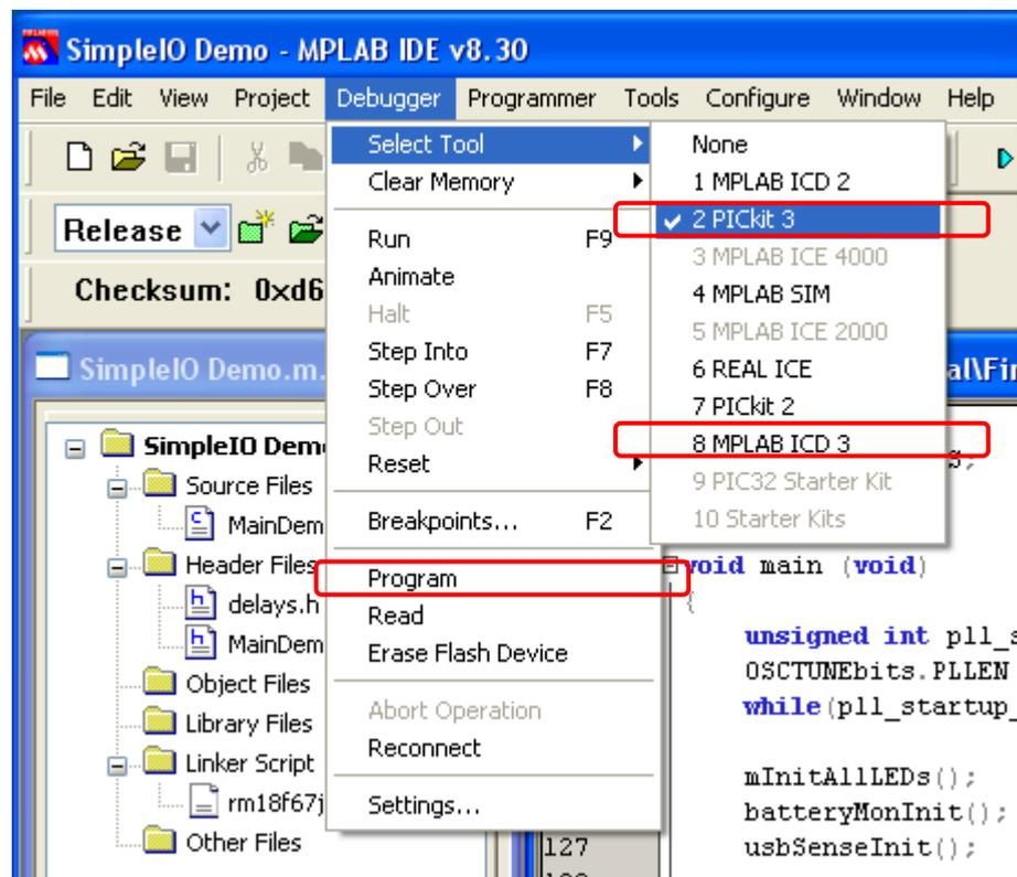
After connection, click *Program*. MPLAB will prompt you for a rebuild. Go ahead to rebuild.
