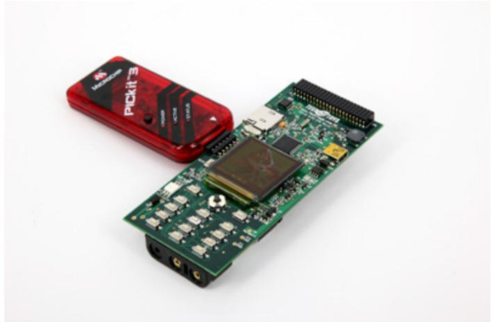
Just in case you would like to use an ICD2/3, a 6-pin 2.54mm ICSP interface is provided.
