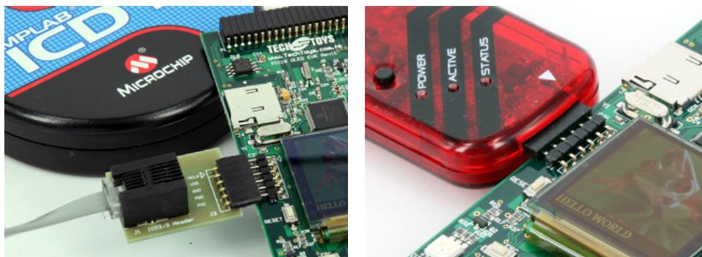
2.2.1.4 Make sure *HIDBootLoader.exe* is not running if you are using a USB cable to supply power to PIC18 OLED EVK kit. For some unknown reason, HID Bootloader connection cannot co-exist with PICKit3. It is either PICKit3 or HID Bootloader connected to the board at any time. Nevertheless, ICD3 does not have such restriction. It is also possible to supply power by batteries, of course. Once “Target Detected” in MPLAB, the Bootloader will be disconnected automatically (see 2.2.1.5 below).
