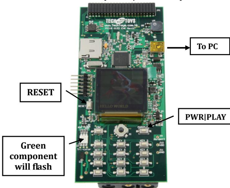
Upon successful connection, the message box of *HIDBootLoader.exe* will show “Device attached” and the green component of the tri-color LED will flash. These are the signatures for a successful connection.
