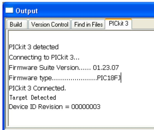
Just in case there is annoying beep from the buzzer upon connection, reboot the MCU by holding **PWR/PLAY** key and then press-&-release **RESET** to bring up the Bootloader firmware. The reason of the beep noise is that the built-in OLED display demo is using pins RB7 and RB6 for keypad. These two pins multiplex with
