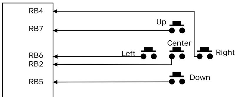
Remarks: keys' pins short to ground to read 0 when pressed
